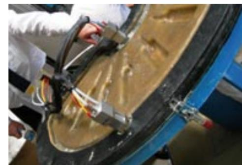
RTM-Light can be used to make small composite parts such as boxes, seats and benches, covers, console supports, etc, but allow also to mould wide deck if moulds are well designed.
