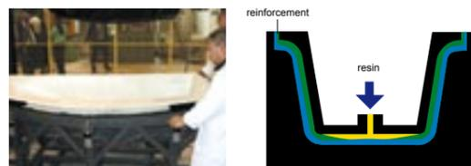
RTM process allows to use filled resin with low shrink additives for an excellent surface appearance of the finished part.
